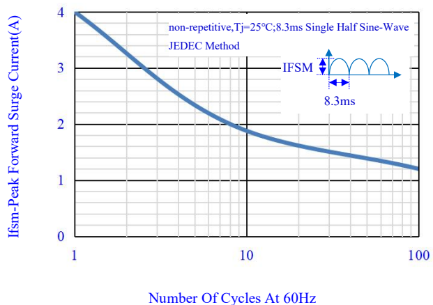
Fig.5-Max. Non-Repetitive Surge Current
